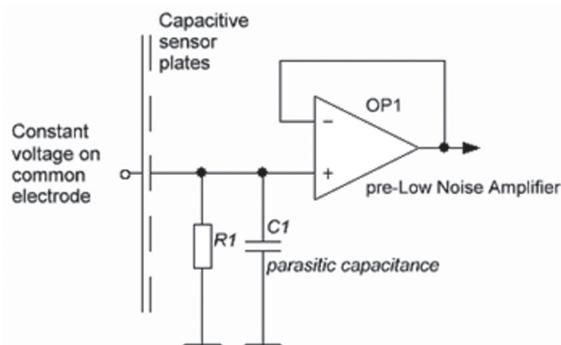
Fig. 1. Principle of reading the signal with RC-sensor
