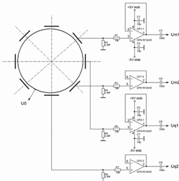
Fig. 2. Simplified block diagram of the electrostatic read out of signals
