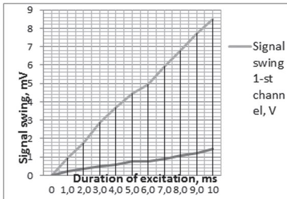
Fig. 5. Dependence the signal swing of the excitation duration. Excitation process in channel No. 1.
