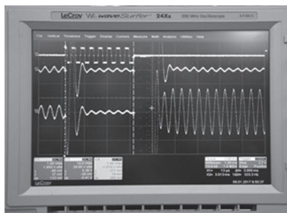
Fig. 4. A typical oscillogram. Blue color — impulses of swing. Green — the output of the main channel Yellow — the output of the quadrature channel
