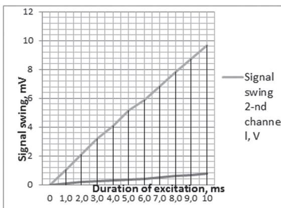
Fig. 7. Dependence the signal swing of the excitation duration. Excitation process in channel No. 2
