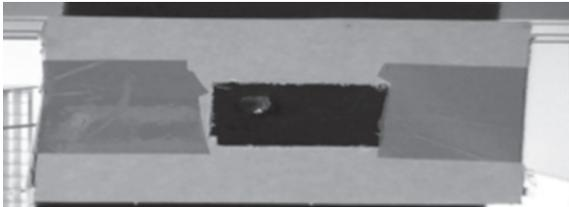
Fig. 12. Measurement configuration which has a hole under the absorber
