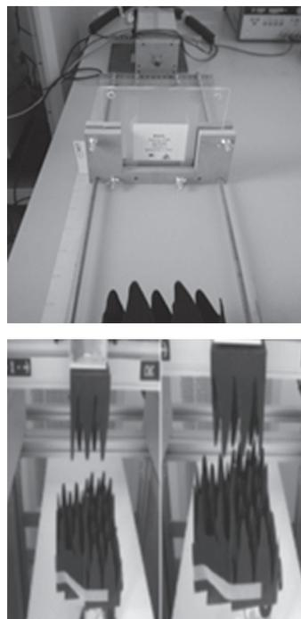
Fig. 20. Setup using plexiglas and PVC sample. Reflection plane is a 6x6 metal plane
