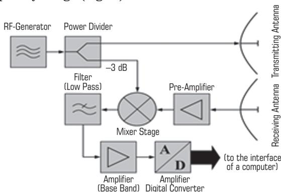
Fig. 1. Microwave part of 3D FMCW terahertz radar
