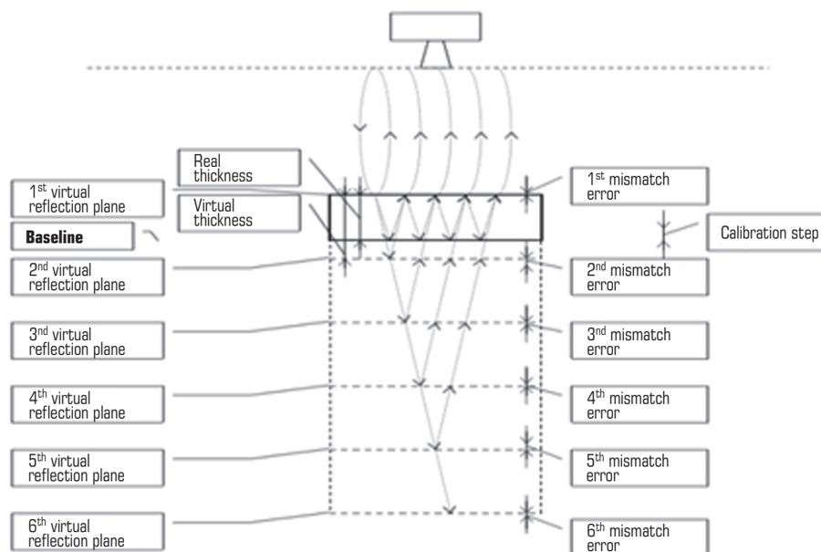
Fig. 3. The reflections of an electromagnetic wave in a plexiglas sample
