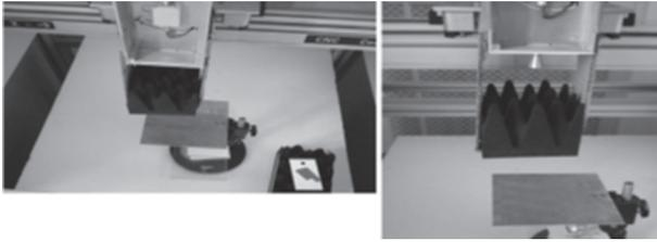
Fig. 11. Measurement configuration with the absorber which has a hole of size of about 1 cm
