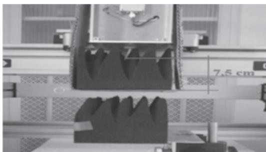
Fig. 5. The configuration of the measurement of a radar system with two absorbers
