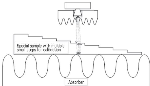
Fig. 4. Calibration of the system using absorber and plexiglas plates of different thicknesses
