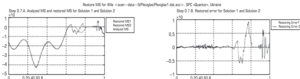
Fig. 28. Attempt to restore source composed MS from calculated distance spectrum
