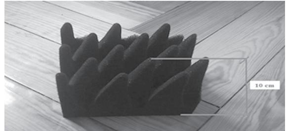
Fig. 16. The absorber for measurement to radar system
