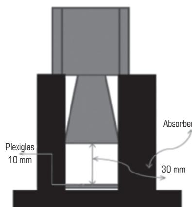
Fig. 2. System for testing 3D radar
