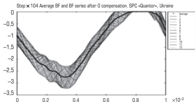
Fig. 24. Comparing of calibration average BF between response signal from absorber only without metal plane and only metal plane
